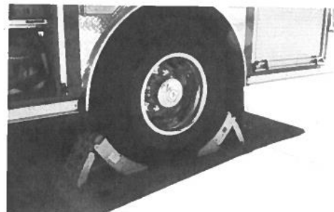
Figure 11.4 The apparatus wheels should be chocked during pumping operations.
